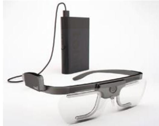
Figure 3: Tobii Pro Eye tracking system
