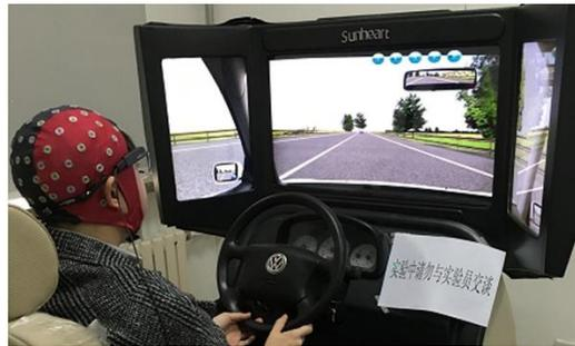
Figure 23: The electroencephalogram (EEG) sensors used for studying drivers' fatigue (Ma et al., 2018)
